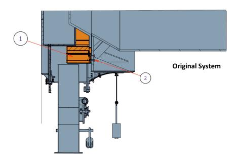
The improvement involves extending the length and the diameter of the current lifter in order to recover and guide as much material as possible back into the process.
